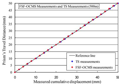
Figure 9: Travel Distances of the Prism and the Corresponding Displacement Measurements.
