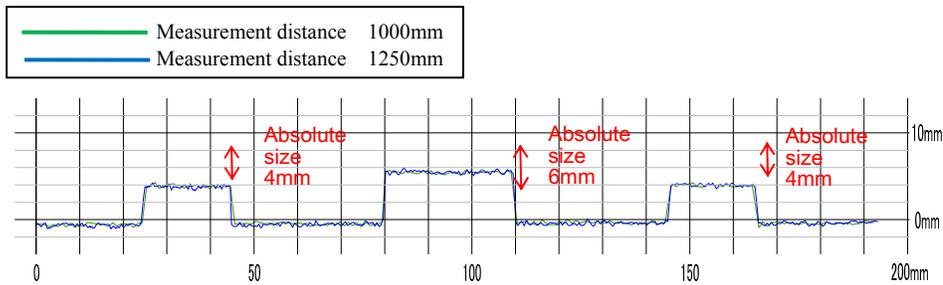
Figure 4: Measurement Results ( A-A section )
