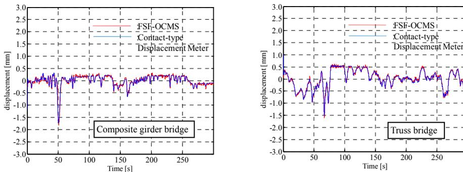
Figure 14: Deflections Measured at the Centers of the Spans of the Girders of the 2 Bridges with Vehicles Traveling over the Bridges
