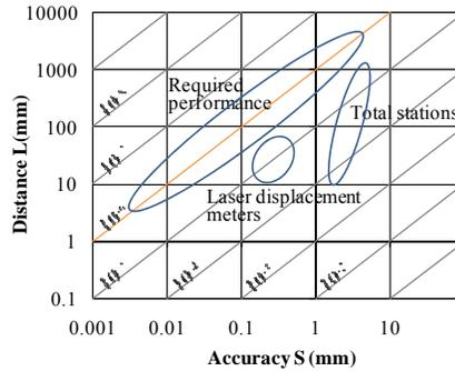
Figure 1: Relationship between the Accuracy and Measurement Distance Requirements in the Construction Field (The figures in the graph are S divided by L.)
