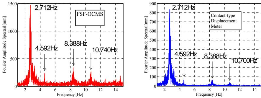
Figure 13: FFT Results (Truss Bridge).
