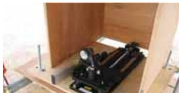
Figure 8: A Prism Target Controlled by high-resolution Position Stage.
