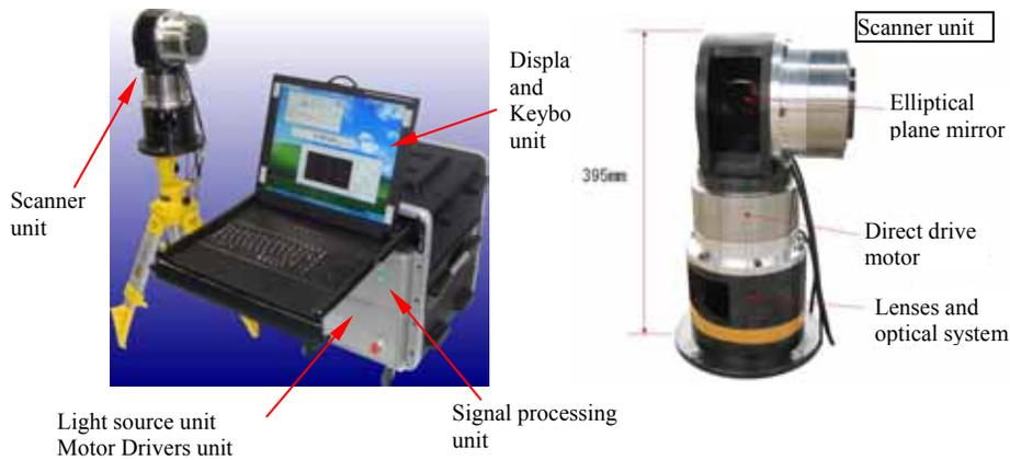
Figure 7: Configuration of the FSF Laser Optical Coordinate Measuring System.
