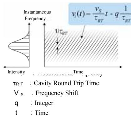
Figure 6: Schematic of a comb chirped frequencies.
