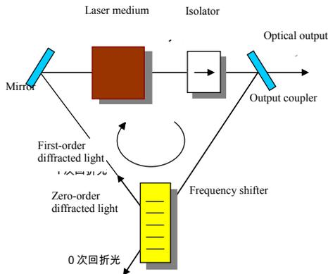
Figure 5: Basic configuration of an FSF laser.
